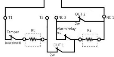
NOTE. In order to use 1<sup>st</sup> way, switches no. 10 (see figure) must be switched to position 4w. In order to use 2<sup>nd</sup> way, switches no. 10 (see figure) must be switched to position 2w.
