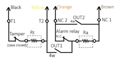
2<sup>nd</sup> way: The actuator TAMPER relay is switched on sequentially with the contacts of the actuator relay contacts. (**Factory settings**)
